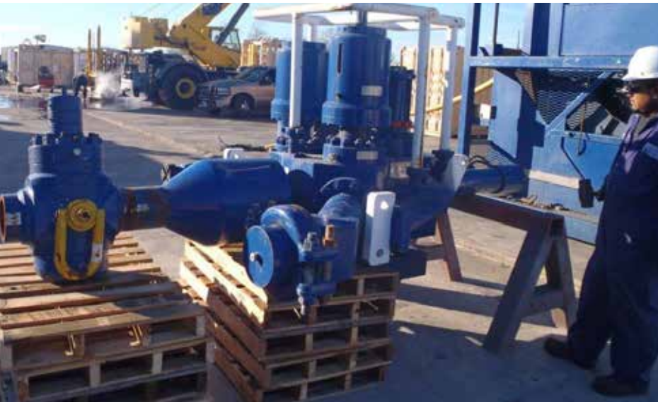
At our subsea facility, WOM employee testing a repaired Flowhead before it goes back to the customer
