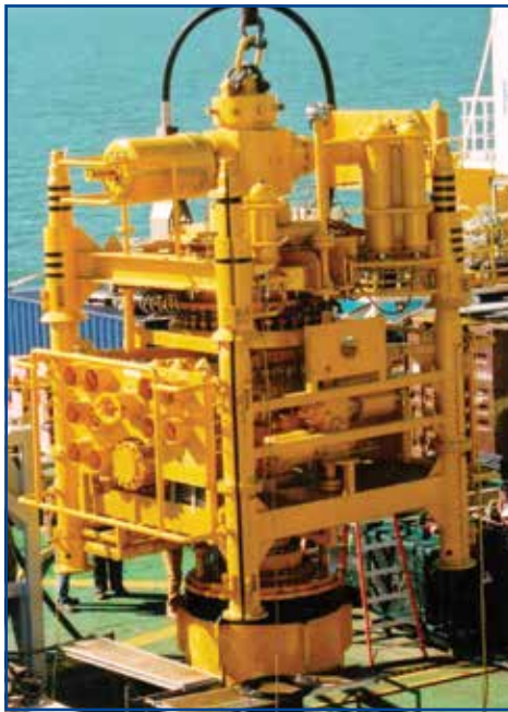
WOM's Subsea Intervention System being deployed on Cal Dive's (Helix) Q-4000
